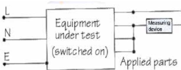
Figure Measurement of patient auxiliary current.
