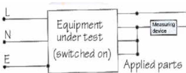
Figure Measurement of patient auxiliary current.
